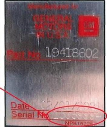
ENGINES ARE FACTORY SEALED - EACH CAP IS RECORDED TO SPECIFIC ENGINE LOCATION MATCHED TO THE ENGINE SERIAL NUMBER: EXAMPLE 15069994. THIS PLATE IS ATTACHED TO THE ENGINE. INFORMATION IS AVAILABLE ONLY TO TECH INSPECTORS FOR TRACK VERIFICATIONS.
